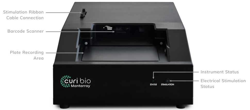
Figure 1: Components and functions of each part of the Mantarray instrument.
