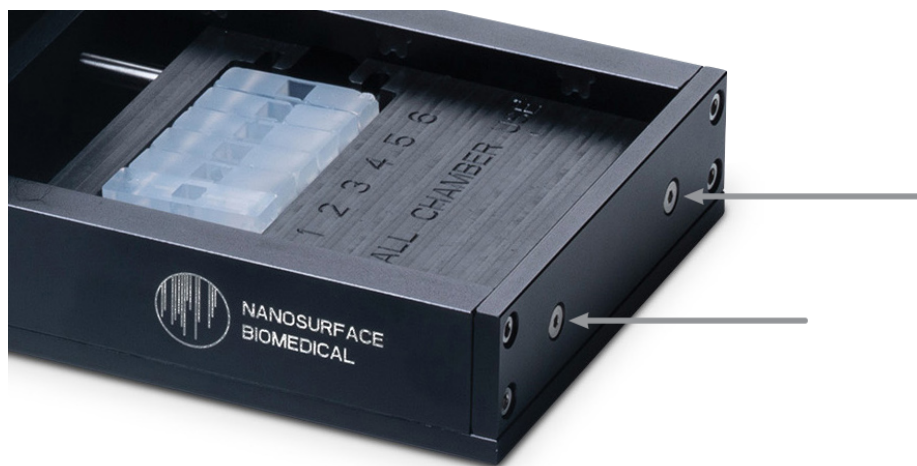
Figure 6: Close-up of the Cytostretcher instrument, with arrows pointing out the two front bolts.
