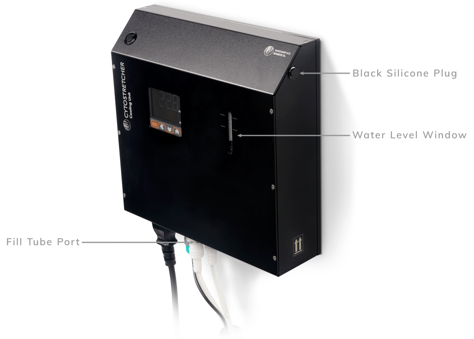
Figure 7: Image of Cooling Unit, referencing specific parts mentioned in the setup process.
