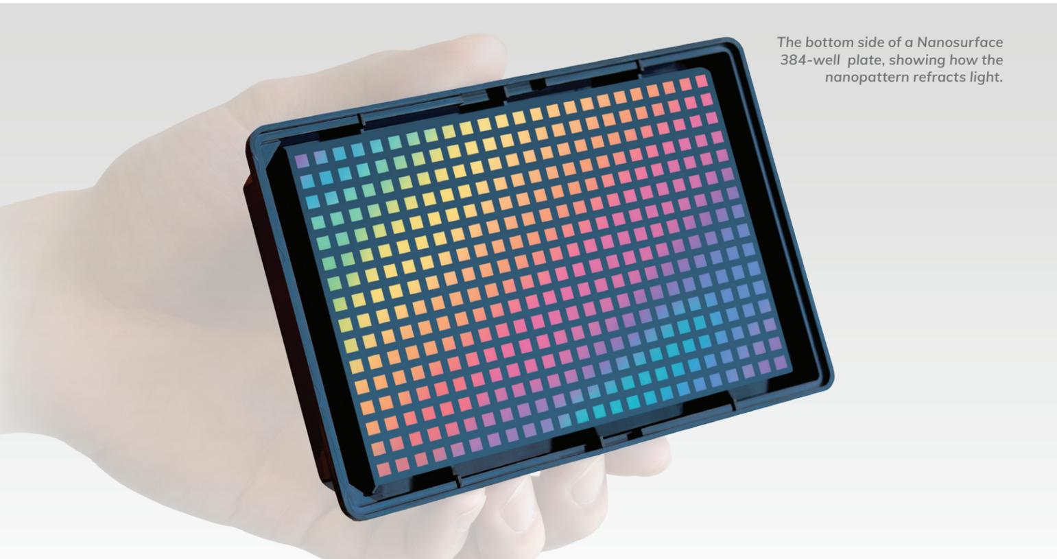
The bottom side of a Nanosurface 384-well plate, showing how the nanopattern refracts light.
